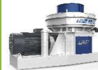
RDF Pelleting Mill
